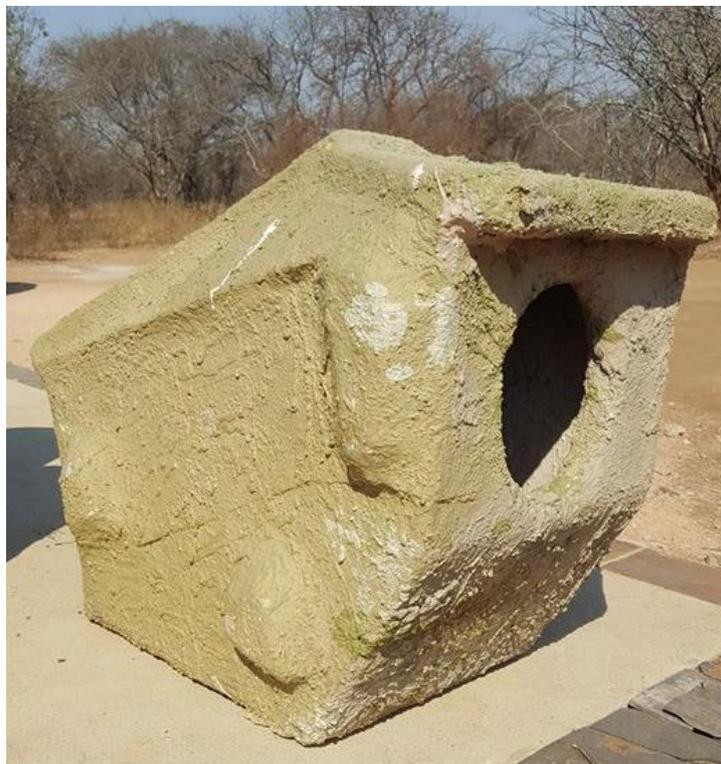
*Figure 4. New nest design made from polystyrene and M1 composite*
